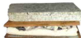
Figure 56.4 Sunmica sheet over wet paste and block of stone over it
