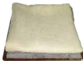
Figure 56.3 Spreading of wet pulp paste on the muslin cloth
