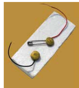
Figure 41.1 A simple switch
