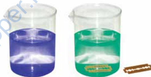
Figure 18.1 Change in colour of the copper sulphate solution due to reaction with iron (shaving blade)
