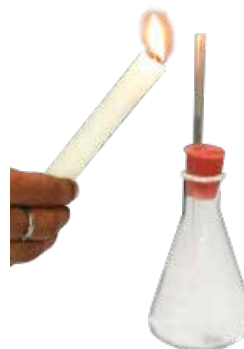
Figure 19.2 Testing hydrogen gas by burning
