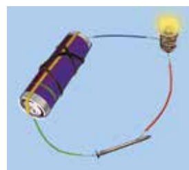
Figure 20.2 Testing whether the bulb glows when the tester is in contact with a iron nail
