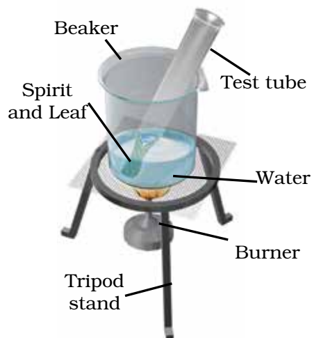
Figure 4.1 Set-up for extraction of chlorophyll
