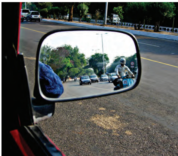
Fig. 11.20 Convex mirror as side view mirror
