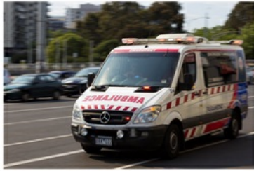
Ambulance is written in reverse, so that a person driving in front can see straight spelling in the rear view mirror and give way.
