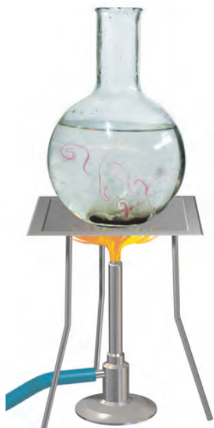
Fig. 3.9 Convection of heat in water
