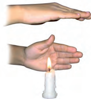
Fig. 3.10 Transfer of heat by convection in air
