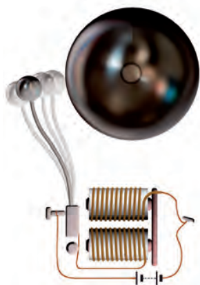
Fig. 10. 20 Circuit of an electric bell
