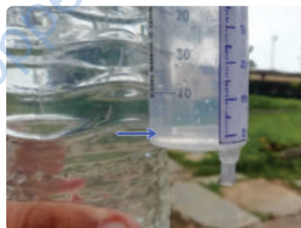
Fig. 7.15 , Fill the measuring unit with water up to '0 mm' before placing the rain gauge model to measure the rainfall.
