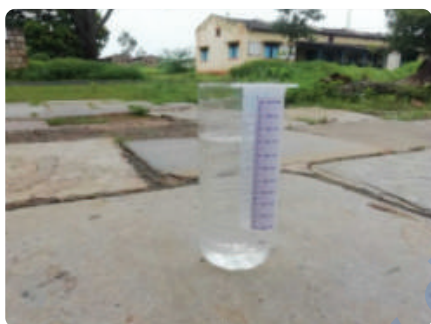
Fig. 7.14 , Mount the measuring unit of the rain gauge on any stand, such as a water-filled container.
