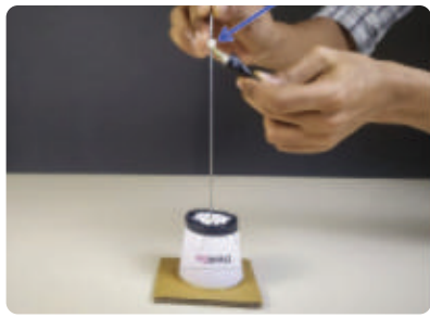
Fig. 7.8, The cycle spoke fixed to a regular paper cup is inserted through a bead. The bead is glued approximately 3 cm from the top of the cycle spoke.
