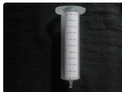
Fig. 7.13 , A millimetre scale template is pasted on the syringe such that the edge with the '0 mm' reading aligns with the edge close to the syringe's tip. The measuring unit of the rain gauge is ready.
