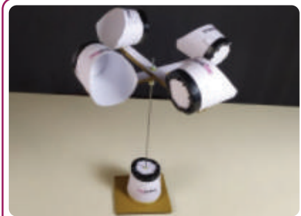
Fig. 7.10, The anemometer model is ready to record wind speed.
