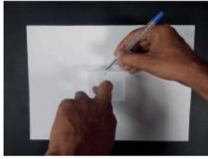
Fig. 5.14 , Place a transparent rectangular container at the centre of an A4 sheet fixed on cardboard & trace its outline
