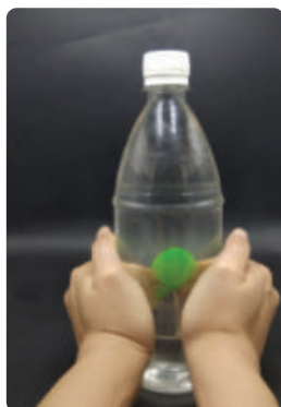
Fig. 5.8, Press the bottle from outside and observe that the balloon contracts a little and the assembly sinks.
