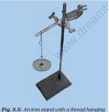
**Fig. 3.5:** An tron stand with a thread hangli from the clamp
