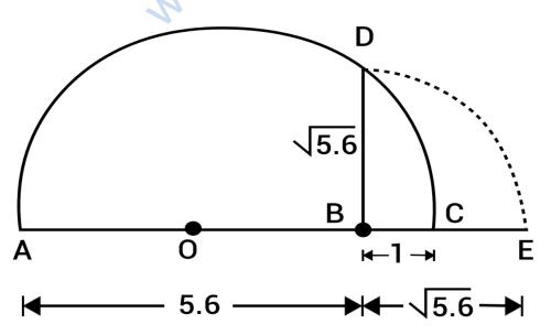
Mark the distance 5.6 units from a fixed point A on a given line to obtain a point B such that AB = 5.6 units. From B, mark a distance of 1 units and mark the new points as C.
