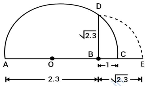
Mark the distance 2.3 units from a fixed point A on a given line to obtain a point B such that AB = 2.3 units. From B, mark a distance of 1 units and mark the new points as C.
