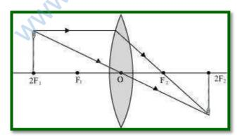
It is given that the image of the needle is formed at a distance of 50 cm from the convex lens. Hence, the needle is placed in front of the lens at a distance of 50 cm.
