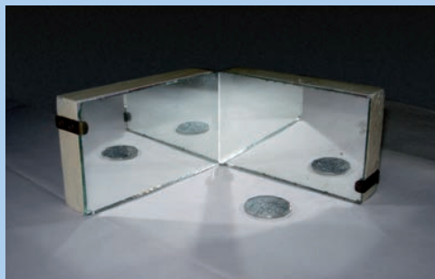
Fig. 13.10 : Images in plane mirror at right angle to each other
