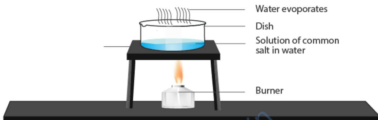
Separation of common salt dissolved in water by evaporation
