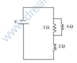
Since, 3  $\Omega$  and 6  $\Omega$  resistors in parallel, so the net resistance
