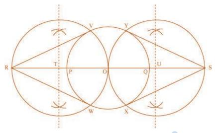
The construction can be justified by proving that RV, RW, SY, and SX are the tangents to the circle (whose centre is O and radius is 3 cm). For this, join OV, OW, OX, and OY.
