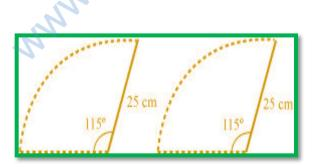
It can be observed from the figure that each blade of wiper will sweep an area of a sector of 115° in a circle of 25 cm radius.
