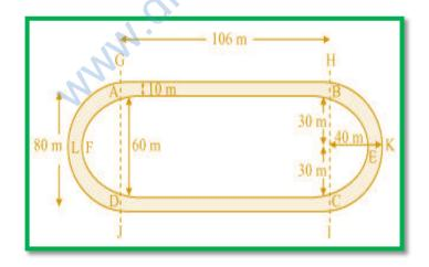
Distance around the track along its inner edge = AB + arc BEC + CD + arc DFA
