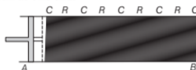
Production of Longitudinal waves in a cylinder by moving a piston back and forth.
