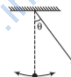
Displacement variable as the deviation of simple pendulum
