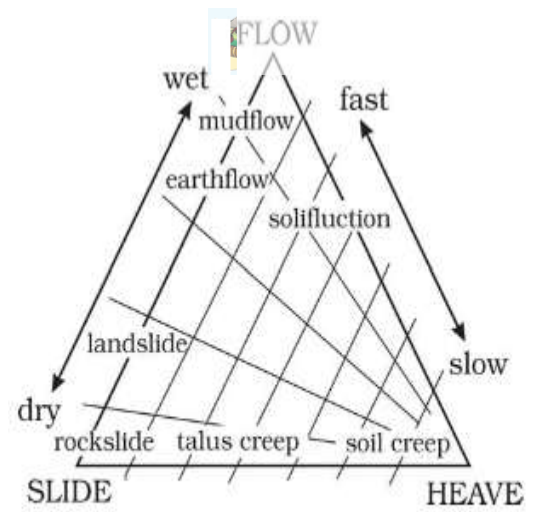
Figure 6.5 : Relationships among different types of mass movements, their relative rates of movement and moisture limits (after Whitehead, 2001)
