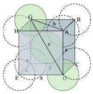
It can be observed from the above figure that the atom at the centre is in contact with the other two atoms diagonally arranged.
