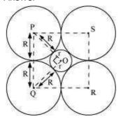
A sphere with centre O, is fitted into the octahedral void as shown in the above figure. It can be observed from the figure that  $\Delta POQ$  is right-angled
