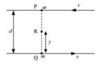
Angular momentum of the system about point P:  $\vec{L}_P = mv \times 0 + mv \times d$ = mvd ... (i)
