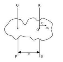
Suppose a rigid body is made up of *n* particles, having masses  $m_1, m_2, m_3, \ldots, m_n$ , at perpendicular distances  $r_1, r_2, r_3, \ldots, r_n$  respectively from the centre of mass O of the rigid body.
