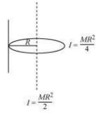
Applying the theorem of parallel axes:
