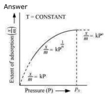
The plot between the extent of adsorption  $\binom{m}{m}$  against the pressure of gas (*P*) at constant temperature (T) is called the adsorption isotherm.
