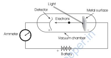
Equipment for studying the photoelectric effect. Light of a particular frequency strikes a clean metal surface inside a vacuum chamber.
