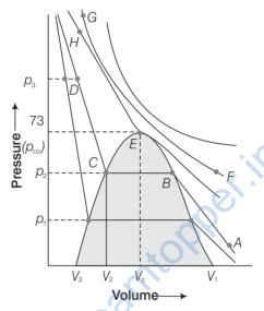
e.g., In figure given above, we can move from A to vertically by increasing the temperature, then we can reach the point by compressing the gas at constant temperature along the isotherm (isotherm at  $31.1^{\circ}$ C). The pressure will increase.
