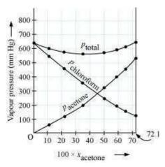
It can be observed from the graph that the plot for the  $p_{\text{total}}$  of the solution curves downwards. Therefore, the solution shows negative deviation from the ideal behaviour.
