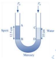
Height of the spirit column,  $h_1 = 12.5 \text{ cm} = 0.125 \text{ m}$ Height of the water column,  $h_2 = 10 \text{ cm} = 0.1 \text{ m}$
