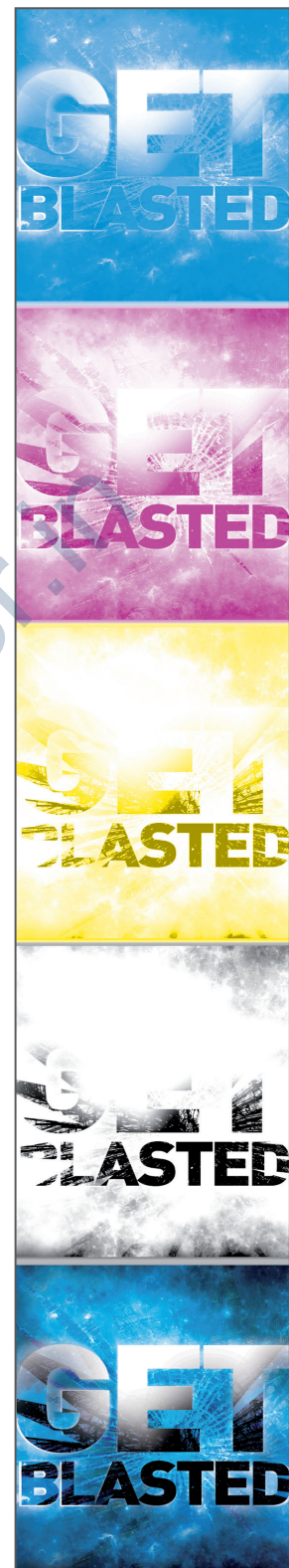
Proofing process with separate CMYK plates
