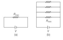
In Fig. (b),  $R_{\rm min}$  provides an equivalent route as in Fig. (a) for current. But in addition there are (n-1) routes by the remaining (n-1) resistors. Current in Fig. (b) is greater than current in Fig. (a). Effective resistance in Fig. (b)  $< R_{\rm min}$ . Second circuit evidently affords a greater resistance.
