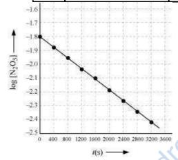
(iv) The given reaction is of the first order as the plot,  $\log[N_2O_5]_{\text{v/s}}$  t, is a straight line. Therefore, the rate law of the reaction is
