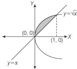
$$\therefore \text{Required area of shaded region, } A = \int_0^1 (\sqrt{x}) dx - \int_0^1 x dx$$
