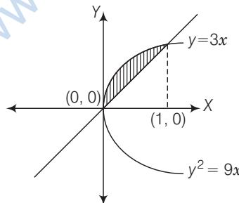
$$\begin{aligned} \therefore \text{Required area, } A &= \int_0^1 \sqrt{9x} dx - \int_0^1 3x dx \\ &= 3 \int_0^1 x^{1/2} dx - 3 \int_0^1 x dx \\ &= 3 \left[ \frac{x^{3/2}}{3/2} \right]_0^1 - 3 \left[ \frac{x^2}{2} \right]_0^1 \\ &= 3 \left( \frac{2}{3} - 0 \right) - 3 \left( \frac{1}{2} - 0 \right) \\ &= 2 - \frac{3}{2} = \frac{1}{2} \text{ sq units} \end{aligned}$$
