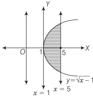
$$\therefore \text{Area of shaded region, } A = \int_1^5 (x-1)^{1/2} dx = \left[ \frac{2 \cdot (x-1)^{3/2}}{3} \right]_1^5 \\ = \left[ \frac{2}{3} \cdot (5-1)^{3/2} - 0 \right] = \frac{16}{3} \text{ sq units}$$
