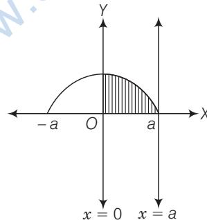
$$\therefore \text{Required area of shaded region, } A = \int_0^a \sqrt{a^2 - x^2} dx \\ = \left[ \frac{x}{2} \sqrt{a^2 - x^2} + \frac{a^2}{2} \sin^{-1} \frac{x}{a} \right]_0^a \\ = \left[ 0 + \frac{a^2}{2} \sin^{-1}(1) - 0 - \frac{a^2}{2} \sin^{-1} 0 \right] \\ = \frac{a^2}{2} \cdot \frac{\pi}{2} = \frac{\pi a^2}{4} \text{ sq units}$$
