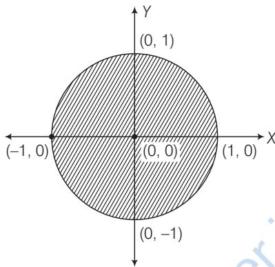
$$\begin{aligned}\therefore \text{Area enclosed by circle} &= 2 \int_{-1}^1 \sqrt{1^2 - x^2} dx = 2 \cdot 2 \int_0^1 \sqrt{1^2 - x^2} dx \\&= 2 \cdot 2 \left[ \frac{x}{2} \sqrt{1^2 - x^2} + \frac{1^2}{2} \sin^{-1} \frac{x}{1} \right]_0^1 \\&= 4 \left[ \frac{1}{2} \cdot 0 + \frac{1}{2} \cdot \frac{\pi}{2} - 0 - \frac{1}{2} \cdot 0 \right] \\&= 4 \cdot \frac{\pi}{4} = \pi \text{ sq units}\end{aligned}$$
