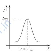
As frequency (v) increases, Z decreases and at certain value of frequency know as resonant frequency  $(v_0)$ , impedance Z is minimum that is  $Z_{\min} = R$  current varies inversely with impedance and at  $Z_{\min}$  current is maximum.
