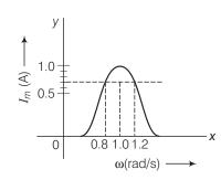
where  $\omega_1$  and  $\omega_2$  corresponds to frequencies at which magnitude of current is  $\frac{1}{\sqrt{2}}$  times of maximum value.
